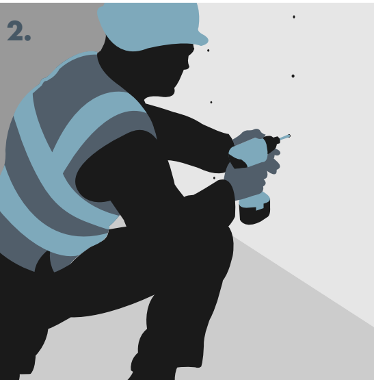
Fixing the boards to the Knauf SFS Studs.
