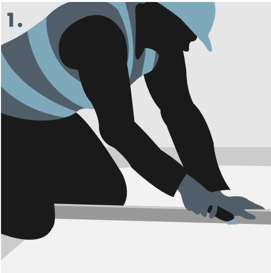
Scoring Knauf Windliner with a knife.
