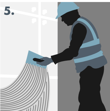
5. Applying notches within basecoat.
