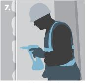
Fixing Knauf Plasterboard onto the Knauf Metal Furring Channel.
