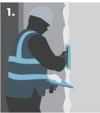
Applying a continuous band of Knauf Plasterboard Adhesive around the perimeter.
