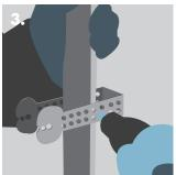
Fixing Knauf 'C' Channel to the Knauf Universal Bracket.
