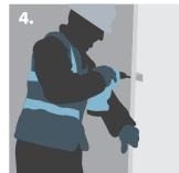
Fixing Knauf Plasterboard to the Knauf 'C' Channel.
