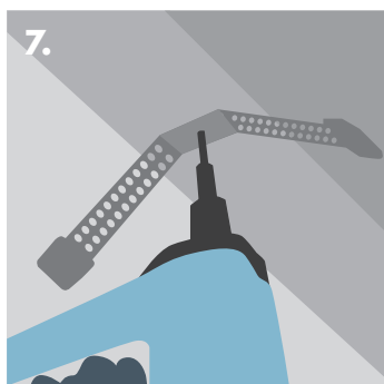
7. Knauf Universal Brackets can be used as an alternative to Knauf Angle Section for shallow voids.
