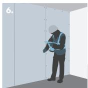
Stagger the boards, to ensure all joints overlap.
