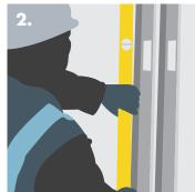
After fixing the head track, the floor track should be positioned by using a vertical stud and a spirit level.
