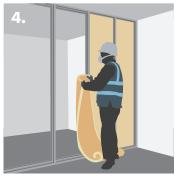
Inserting Knauf insulation quilt between the Knauf 'C' or 'I' Studs.
