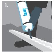
Applying continuous beads of Knauf Sealant to perimeter framing.
