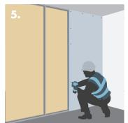
Fixing Knauf Plasterboard to the Knauf 'C' or 'l' Studs.
