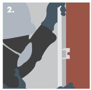
Pushing Knauf 'C' Channel into the Knauf Fixing Clips.
