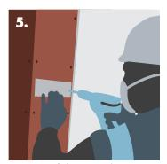
Fixing Knauf Flat Fixing Plate between layers.
