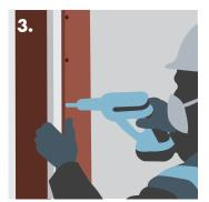
Fixing Knauf Fire Panel onto the Knauf 'C' Channels.
