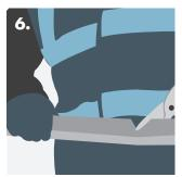
Snip and bend Knauf 'U' Channel to form door head.
