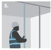
Inserting timber ground into jamb stud door opening.
