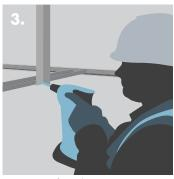
Fixing Knauf Angle Section to upper Knauf 'C' Channel.
