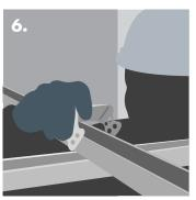
Connecting lower and upper Knauf 'C' Channel with Knauf Channel Intersection Connectors.
