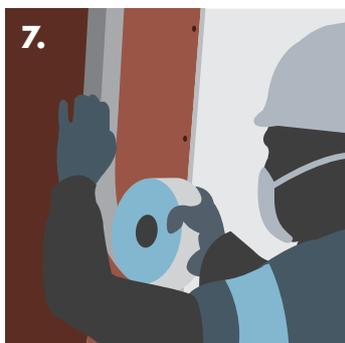
7. Taping and jointing encasement corners
