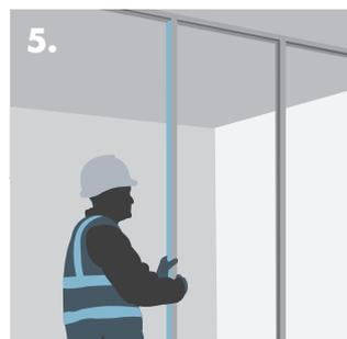
5. Inserting timber ground into jamb stud door opening.
