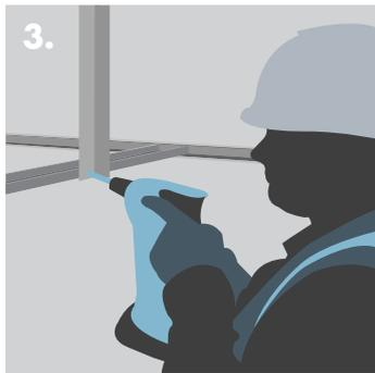
3. Fixing Knauf Angle Section to upper Knauf 'C' Channel.
