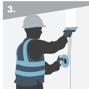
3. Embedding Knauf Aquapanel Exterior Joint Tape.
