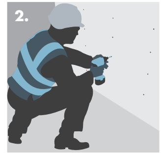
2. Fixing the boards to the background members.
