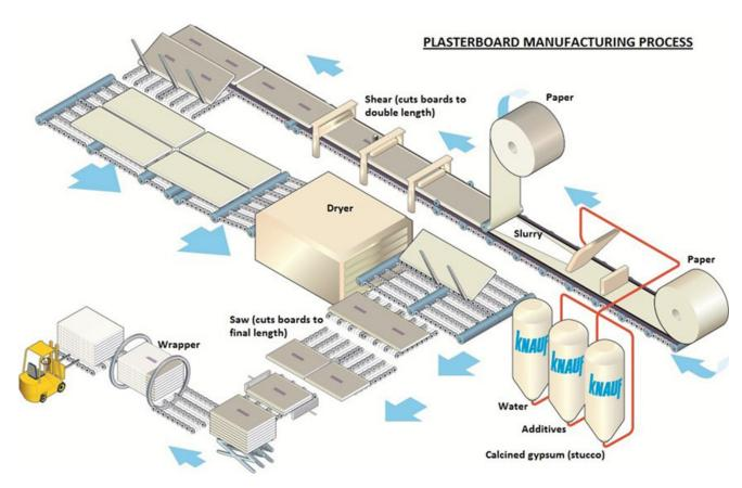
Raw materials are homogeneously mixed to form a gypsum slurry that is spread via hose outlets onto a paper liner on a moving belt conveyor. A second paper line is fed onto the production line from above to form the plasterboard. The plasterboard continues along the production line where it is finished, dried and cut to size.
