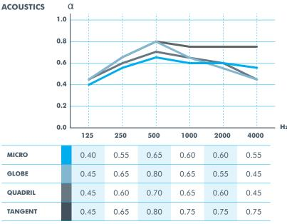
CONSTRUCTION 200 mm suspension, no mineral wool
