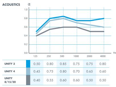
**CONSTRUCTION** 200 mm suspension, no mineral wool
