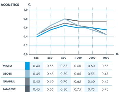
**CONSTRUCTION** 200 mm suspension, no mineral wool
