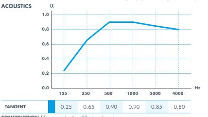
**CONSTRUCTION** 55 mm construction, 33 mineral wool
