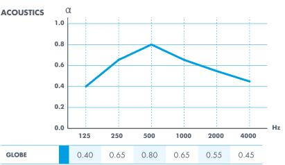
**CONSTRUCTION** 200 mm suspension, no mineral wool
