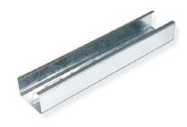
Knauf Acoustic C Studs are galvanised lightweight steel sections for use in non-load bearing Knauf partition systems, specifically designed to improve the acoustic performance of the resulting partition. A 50mm flange makes it ideal for use in conjunction with Knauf AQUAPANEL® Indoor.
