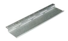
Knauf Resilient Bar is a resilient metal section which is fixed to the underside of floor joists and to the face of partitions to reduce direct sound transmission.
