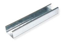
Knauf Acoustic C Studs are galvanised lightweight steel sections for use in non-load bearing Knauf partition systems, specifically designed to improve the acoustic performance of the resulting partition. A 50mm flange makes it ideal for use in conjunction with Knauf AQUAPANEL® Indoor.
