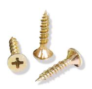
AQUAPANEL® Maxi Screws have been specially developed for fixing AQUAPANEL® Cement Board on to timber and metal frameworks of differing thicknesses. Both countersunk needlepoint and countersunk drillpoint versions are available. AQUAPANEL® Maxi Screws can be used for both wall and ceiling applications in interior and exterior applications.
